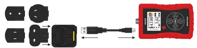
The unit should reach full charge within 4 hours. The battery status icon will indicate charging is in progress (see 6. *Display & 8. Battery status*).
