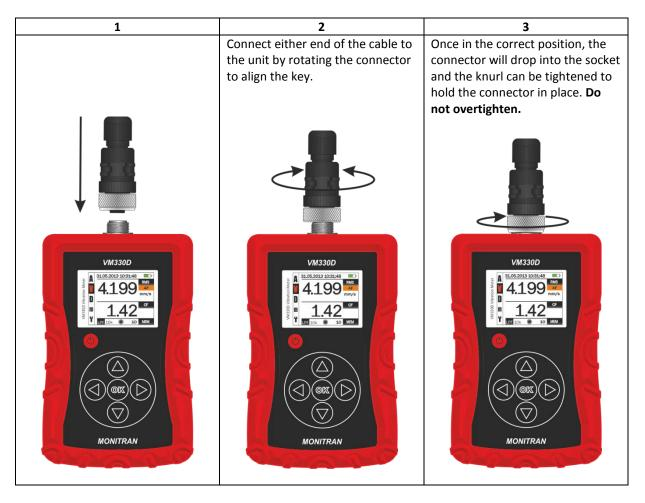
• Repeat this process to connect the sensor to the other end of the cable.
